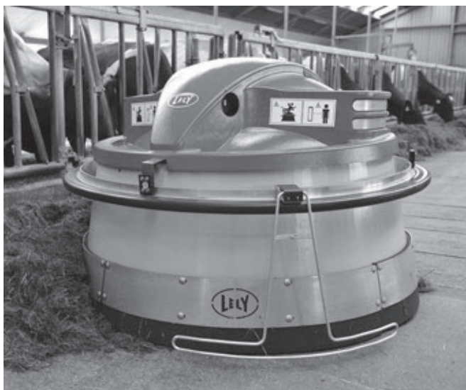
Cows on robot-equipped farms are usually kept in all year round, giving rise to the need for another robot, which moves up and down the aisle ensuring that silage is within reach of the stalled cows.
