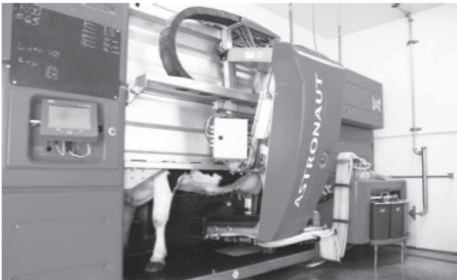
Spot the cow. The Dutch made Lely Astronaut is the leading make of robot milking machine.
